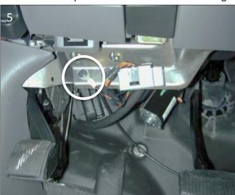
5. Strip and twist together the ends of the black wires from each extension wires. Crimp them together in the supplied ring connector. A good ground location is located on the bare metal under the dash just below and left of the steering plate behind the hood release lever. Verify the turn signal working properly before replacing any trim pieces, door panels, plastic moldings to finish installation.
