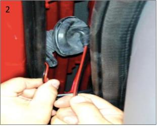
3. The electrical wiring for the turn signals is located just below and left of the steering column. Locate the GREEN WITH WHITE STRIPE wire from within the wire bundle. Turn the ignition key so that electrical power is on and activate the driver side turn signal. Probe the wire with the wire tester to verify that flashing turn signal power is present. This is your driver side turn signal wire(+). Then, locate the WHITE WITH BLUE STRIPE wire from within the wire bundle. Activate the passenger
